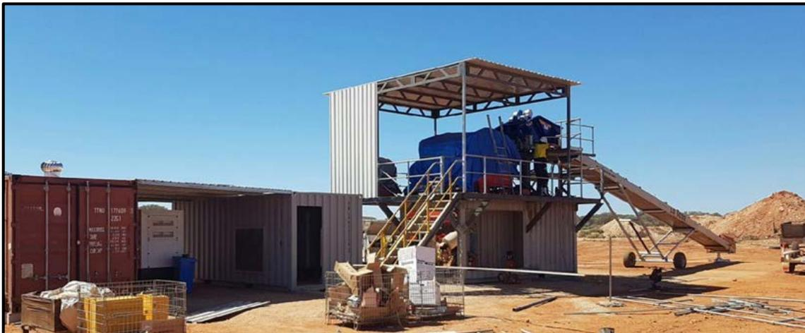
**Figure 2: Ore Sorting Platform with feed conveyor and roofing installed.**
