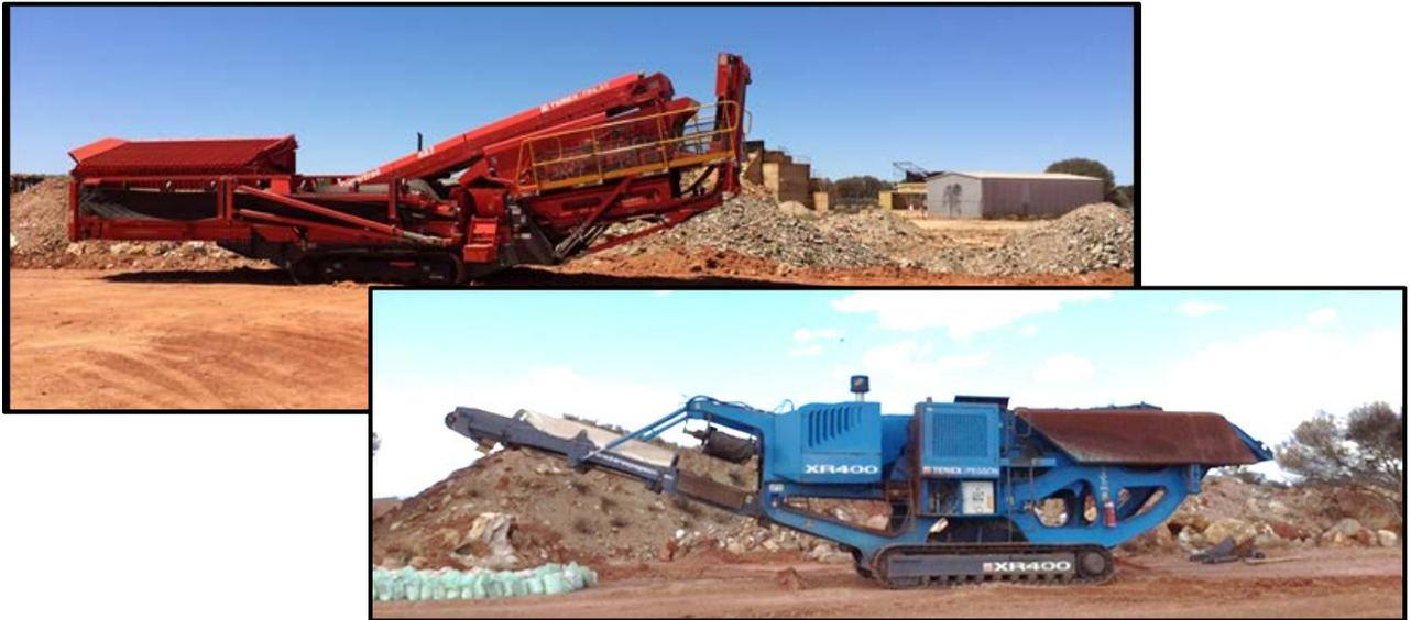
**Figure 2: Mobile Crushing and Screening plants**
