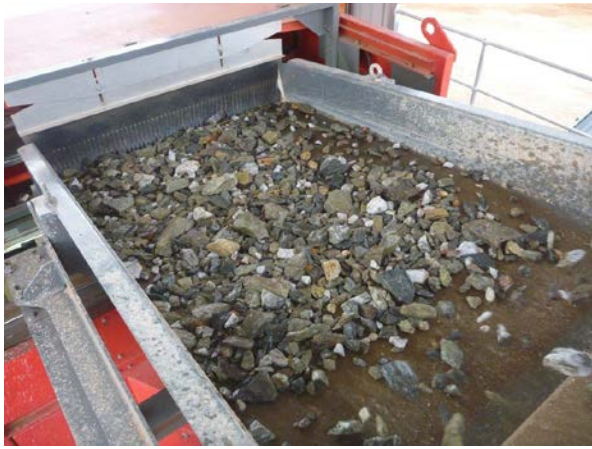
Figure 3: Feed material presented to the sorter
