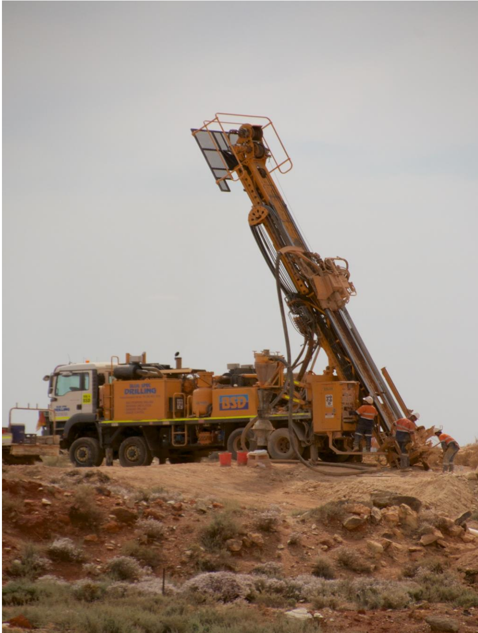
Photo 1: Diamond Drill Rig on Site at Second Fortune
